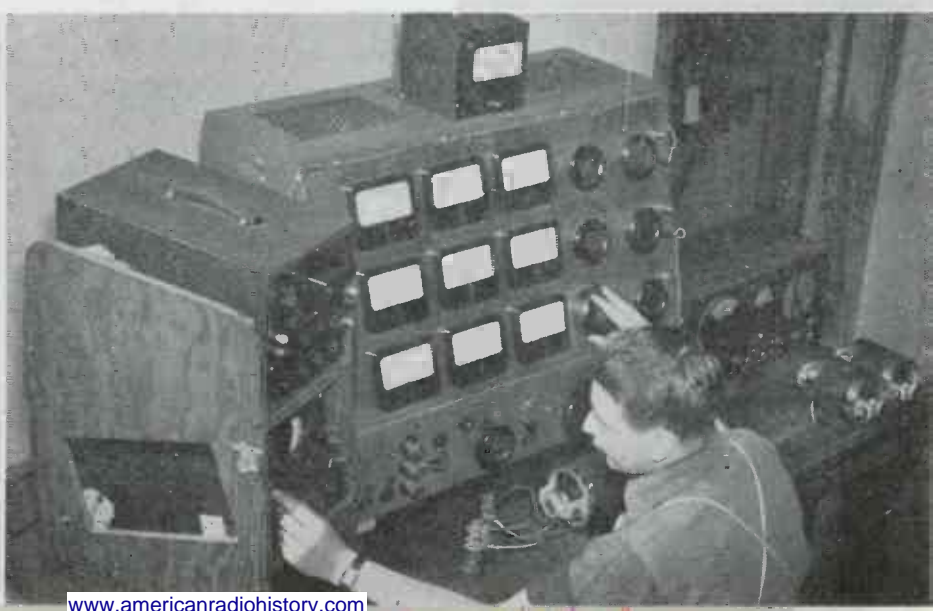
9 —Well built custom designed test jig permits rapid testing of many properties of dynamotors coming off production line at ▼ Carter Motor Company, Chicago, Ill.
