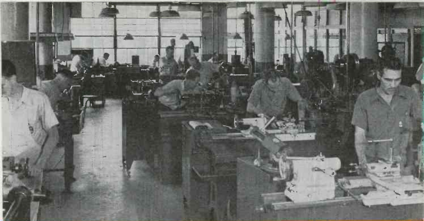
The engineering model shop, of which this is a portion, is fully equipped with modern machine tools for the pilot production of war and postwar equipment
