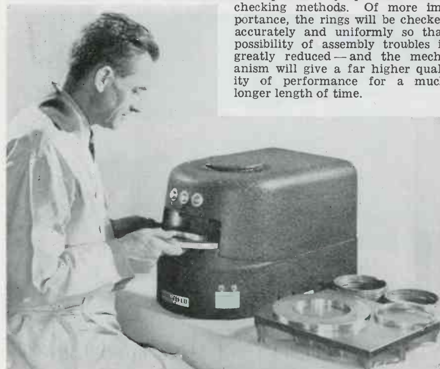
The electronic piston ring inspector, depending for operation upon photoelectric tubes reduces inspection time per piece to five seconds, greatly improves accuracy
