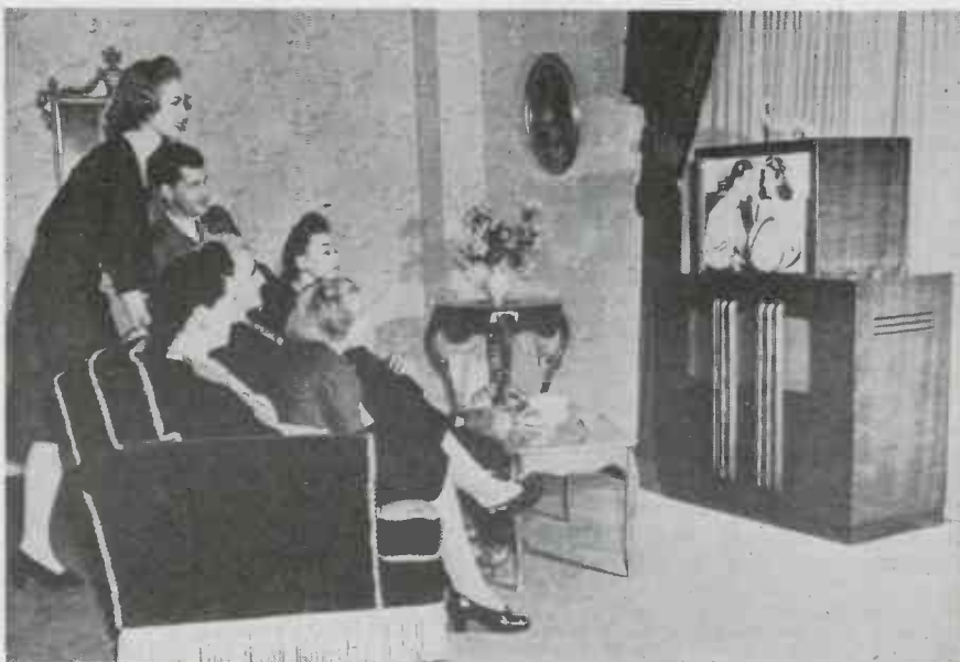
The advance development model of the new RCA projection type home television receiver is equipped with a translucent viewing screen measuring 21 1/3 by 16 inches
