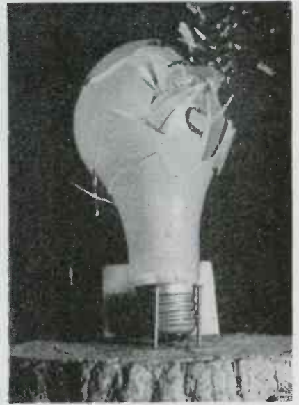
These two photographs were made by Arthur Palme, Pittsfield, Mass., with a home-made variation of the Speedlight originally developed by Professor Harold E. Edgerton of MIT. In both cases the damage was done with a 22 cal. rifle, the lamp bulb photo being made at 1/15,000th second and the teacup at 1/10,000th second
