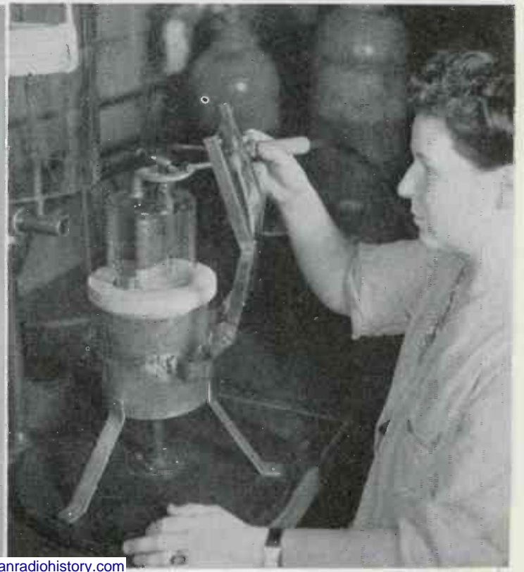
5 —Brazing technique is applied in fastening plate connector to the cap on 833A transmitting tubes at North American Philips Co., Inc. Operator is protected from tube shattering by plastic screen.
