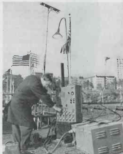
When the old ball season opens WNBT may likely again set up a remote pickup like this to relay the games to its transmitter located atop the Empire State Building in New York
